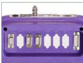
D-SUB connectors - IP40
